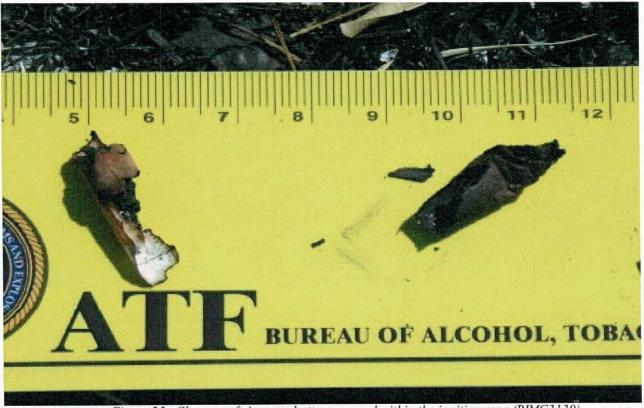
Figure 25: Close-up of cigarette butts recovered within the ignition area (RIMG3139)
