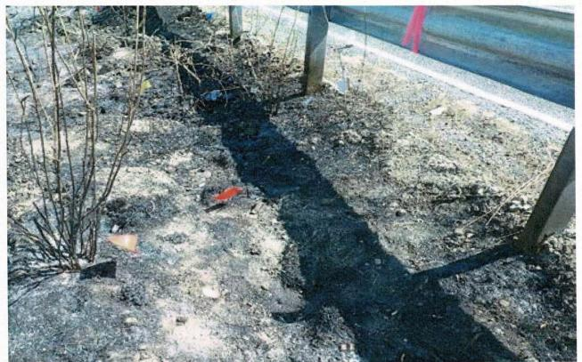
Figure 23: Identified Ignition Area marked with white flags and below the pink flagging tape (RIMG3128)
